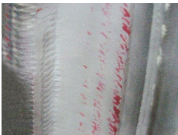
Fig. 5 Liquid penetrant indications of 52M hot cracks welded on an ER308L buffer layer deposited on CF8A base metal of similar composition to the cast pipe in the plant
