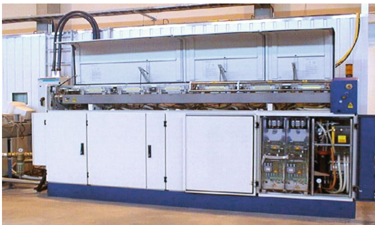
Fig. 6 3 kW Nd:YAG-laser used in the experiments
